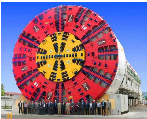
Tunnel excavator for building underground base
